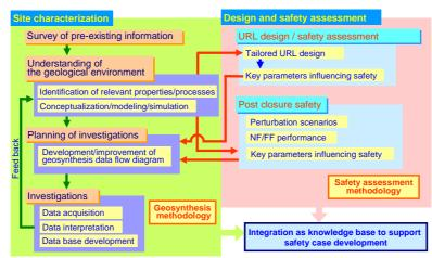
Figure 5. Conceptual data flow diagram and framework for safety case development (after Hatanaka *et al.*)
